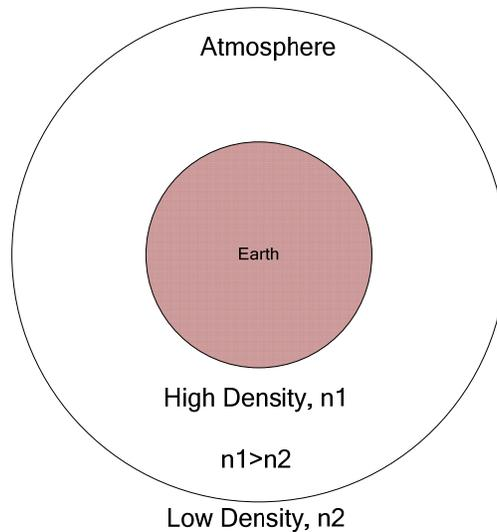
Thus, the refraction index ( $n$ ) will also change. As a consequence, a ray sent from one antenna tends to follow the earth surface. It is a very small variation, but sufficient to help microwave engineers to reach unseen sites. The end result is that the earth can be considered a little bit flatter. The bulge of the earth for a standard atmosphere can now be calculated:
